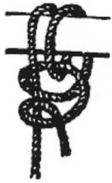
Fisherman's Bend for fastening rope to a ring or anchor.
