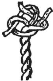
Wall Knot to prevent unstranding and act as a stopper.
