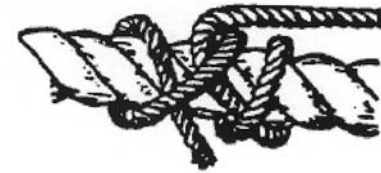
Rolling Hitch for hauling spar or large cable.
